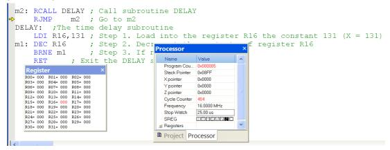
Fig. 5. AVR Studio environment window in debug mode of DELAY subroutine
